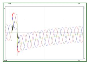
Fig. 4. Oscillogram of phase-to-ground and neutral-to-ground voltages at an arcing ground fault in 6 kV network with ungrounded neutral (I<sub>fault</sub>=10.75 A)
