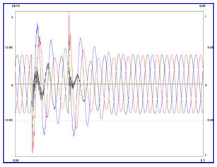
Fig. 9. Oscillogram of phase-to-ground and neutral-to-ground voltages at an arcing ground fault in 10 kV network with a neutral connected to ground through a ground fault neutralizer in parallel with a resistor
