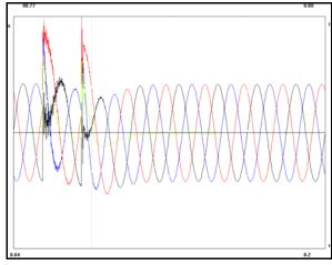
Fig. 10. Oscillogram of phase-to-ground and neutral-to-ground voltages at an arcing ground fault in 35 kV network with a neutral connected to ground through the 8000-Ohm resistor
