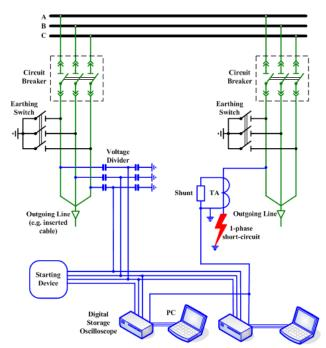
Fig. 1. Connection diagram of measuring equipment at capacitance current measurement and registration of transient process at single phase-to-ground fault
