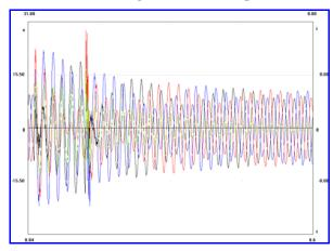
Fig. 5. Oscillogram of phase-to-ground and neutral-to-ground voltages at an arcing ground fault in  $10 \, kV$  network with resonant grounded neutral through ground fault neutralizer ( $I_{fault} = 61.3 \, A$ ,  $I_{GFN} = 77 \, A$ , overcompensation is 25%)
