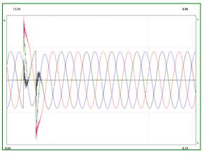
Fig. 8. Oscillogram of phase-to-ground and neutral-to-ground voltages at an arcing ground fault in 6 kV network with a neutral connected to ground through the 400-Ohm resistor
